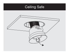
Remove module holder with suction cup for LED module replacement / maintenance.
