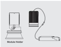
4. Attach module to module holder 5. Adjust the angle required. with spring clip and connect module to driver.
