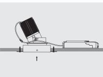
6. Gently insert module holder from the bottom of the fixture frame to complete installation.
